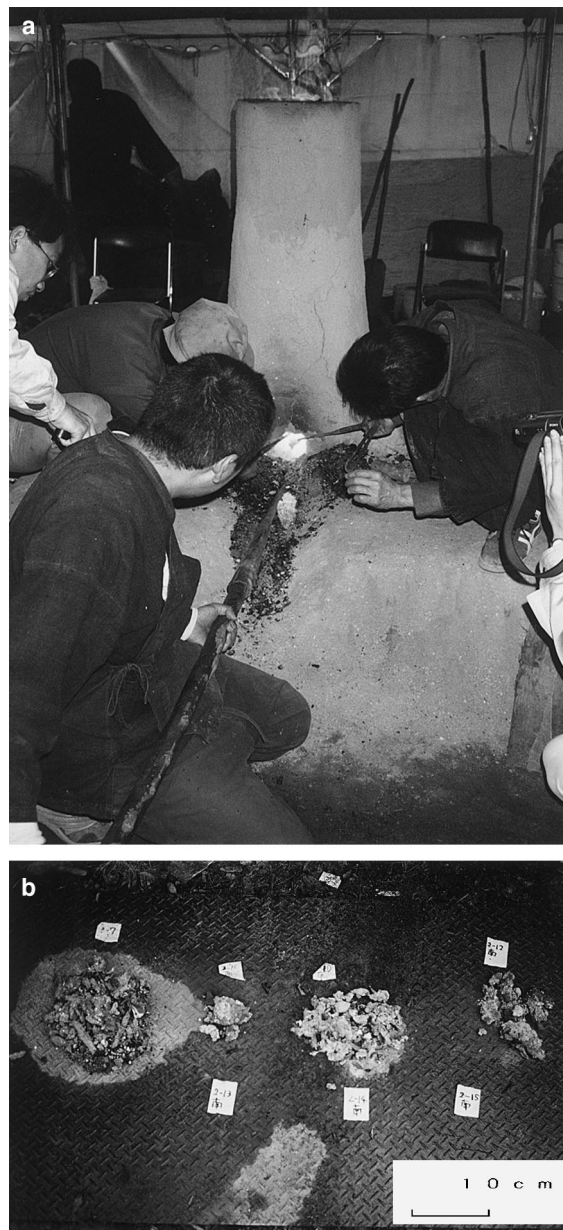
Fig. 1. (a) Raking the slag from the iron manufacturing furnace in the reproducing experiment of ancient iron manufacturing. (b) The slag from iron manufacturing process. With the progress of the process, the ingredient changes.
